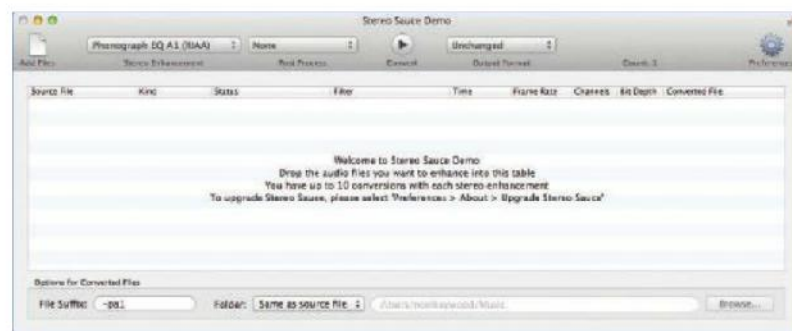
The user interface is stark, but simple. Add File at top left loads a digital file, you select a process then press the central Play button. The file is then altered accordingly – a new, updated version being generated.
